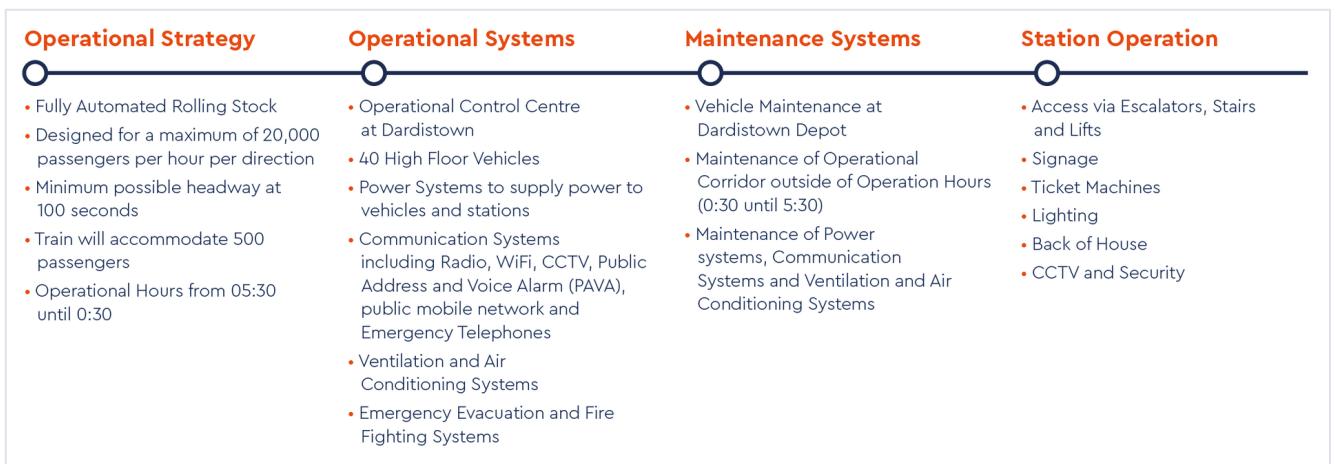
Diagram 1.3: Summary of Key Activities during the Operation Phase of the Proposed Project
